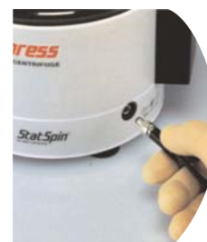
The 24V line to the centrifuge includes a locking nut for secure installation.
